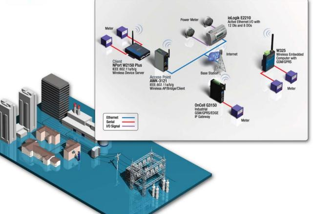
Industrial Networking Applications > Automatic Meter Reading
